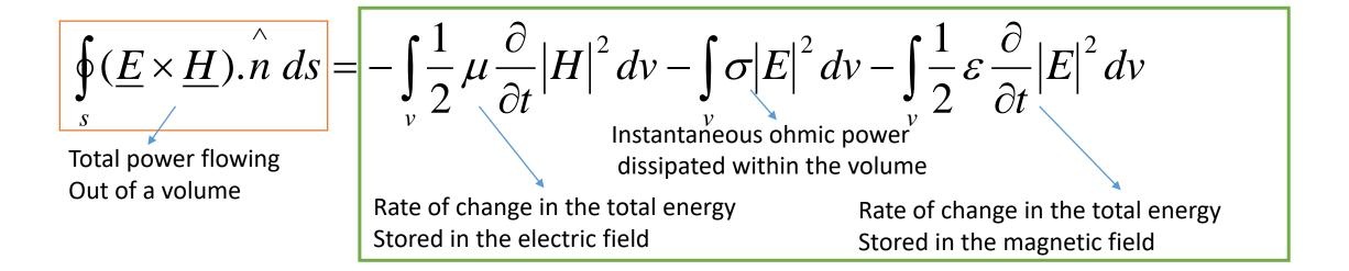
Power *leaving* the volume V enclosed by S= Decreasing electric and magnetic power- Dissipating ohmic power
